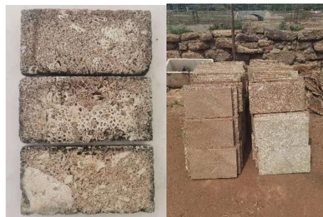
Fig. 1. Existing coral stone brick in the courtyard.
