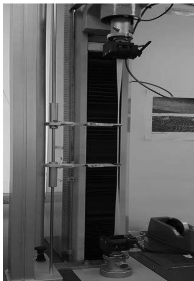
Figure 0.32 Elongation of samples during tensile strength test
