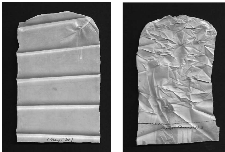
Figure 0.29: Standardized folding method (Left) and non-uniform crumpling method (Right)
