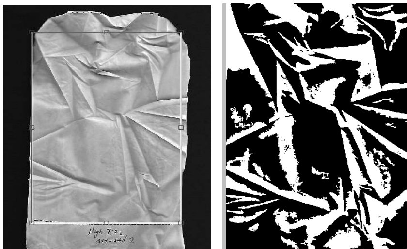
Figure 0.30: Selection of measurement area (Blue box) for MATLAB (left) Contrasting of scanned image (right)
