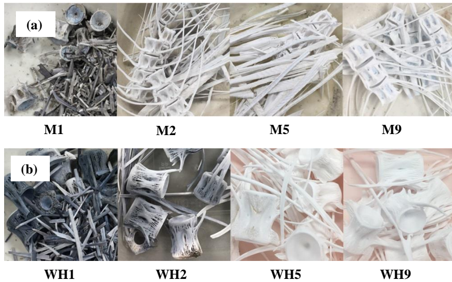
Fig. 2. Changes of bones color due to calcination temperature and time for (a) WWH and (b) SM from temperature (left to right): 400°C, 2 hrs; 600°C, 2 hrs; 800°C, 4 hrs and 1000°C, 6 hrs.
