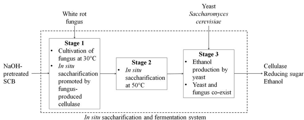
Fig. 1. Experimental procedures of the *in situ* saccharification and fermentation system.
