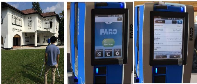
Fig. 3. The setting up of laser scanner and placing of laser scanner reference spheres and the user interface of the 3D laser scanner.
