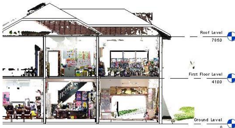
Fig. 6. The datum such as the floor levels and grid was determined and shown in the section view.
