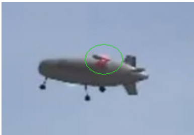
Figure 7 XPLANE cruise/plane control mode with 0° thrust position
